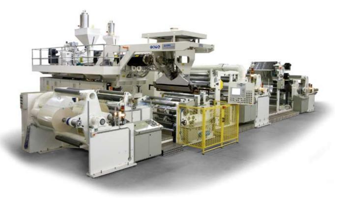
Colines<sup>®</sup> recently took part with the company Alcat to the realization of an extrusion coating line meant for the production of champagne caps. It is a project of remarkable success for a line producing with a max. mechanical speed of 250 m/min and with a max. production speed of 220 m/min; the band is 1.350 mm wide and the thickness of the extruded film is included between 10 and 80 g/m<sup>2</sup>. The extrud-
