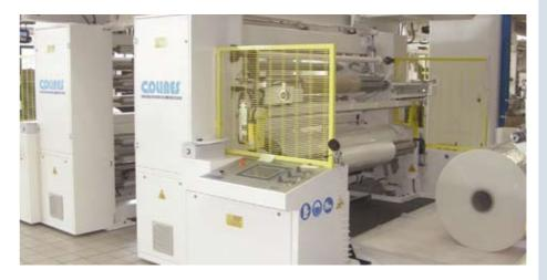
It is already in production and can be seen in Open House at the facilities of our sister company B-Pack<sup>®</sup> spa the new Barrierblown<sup>®</sup> line, with a useful width of 1800 mm for the manufacturing of 5-layers barrier film.
