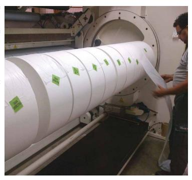
On this line **COLINES**® has also introduced for the first time the new independent rotary axis winder, called **FLEXIWIND**®, which permits to wind-up flawlessly as much as 11 reels 200 mm wide with a perfect geometry and with no tail at the mentioned speed and throughput levels. Furthermore, this winder is equipped with "reverse" technology, which allows to wind up the film in both directions, and can make reels up to a diameter of 1200 mm.
